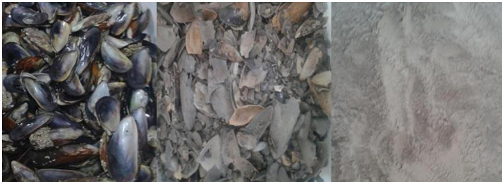
Fig 3: Appearance of mussel shells before and after treatment and grinding.
