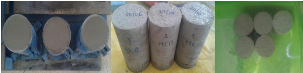
Fig 4: Molding, demolding, and curing of specimens.
